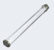
EVF-P lighting fixtures are manufactured with an high resistance cylindrical polycarbonate lamp housing and with end cups made of corrosion resistant copper free aluminium. Polycarbonate lamp housing is a three layers-extrusion UV resistant able to grant the best protection against sun rays and related yellowing effect.
